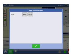
3. If the pump is in Agitate mode, the button will be greyed out. To stop agitation, press the *Agitate* button again.
