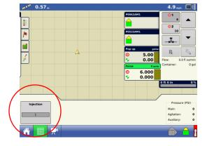
2. Press on *Prime* to prime the injection pump or *Agitate* to agitate the liquid.
