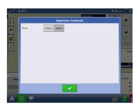
To prime, press the *Prime* button. The pump will run for 3 minutes. Press the *up* and down arrows to vary pump speed.
